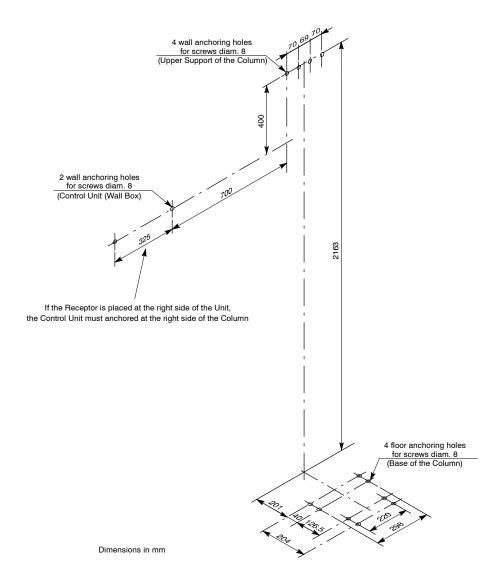
6. Position the Column and make it firm to floor and wall. Check that it is properly levelled on both lateral sides and on the front. Make sure the Column is firmly anchored. (*Refer to Illustration 3-3*.)
