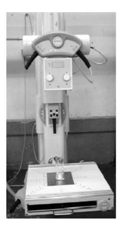
Turn on Collimator light and center the Collimator in relation to the Bucky Table-Top. Horizontal and transversal position of the light axes projected by the Collimator Lamp must be in line with the axes or film sizes marked on the Table-Top.
