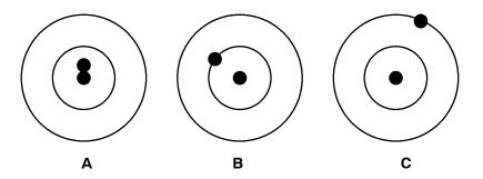
c. Check that the X-ray Beam is properly centered with the Image Receptor. To determine the center of the Image Receptor, draw diagonal lines from corner to corner of the X-ray Film. (Alternately, the film can be folded in half and creased at the center). The two lines will cross in the center of the Image Receptor (film). Then draw diagonal lines from the corners of the imaged X-ray Field.
