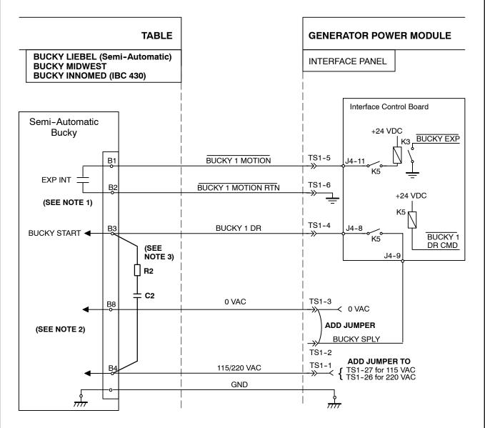
NOTE 1: Be sure that B2 terminal is not connected to B3 terminal.
