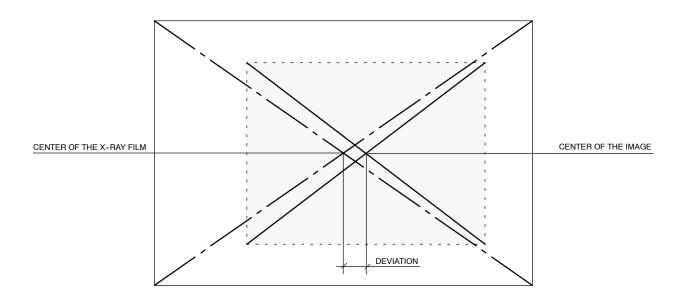
If the deviation is greater than 2% of SID, perform the following procedure:
