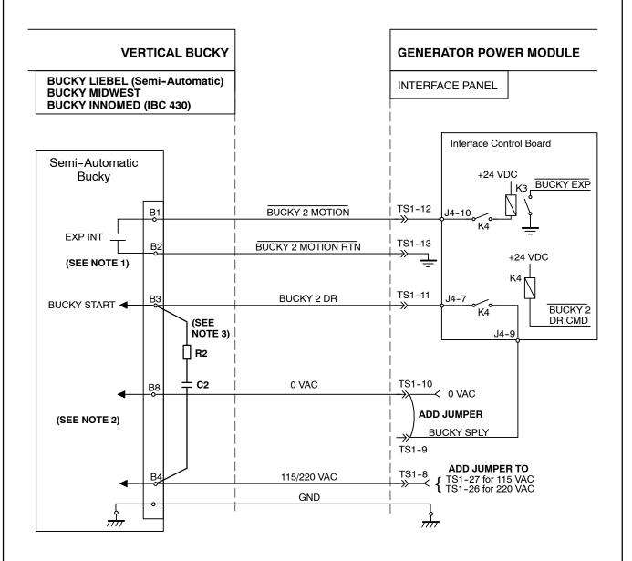
NOTE 1: Be sure that B2 terminal is not connected to B3 terminal.
