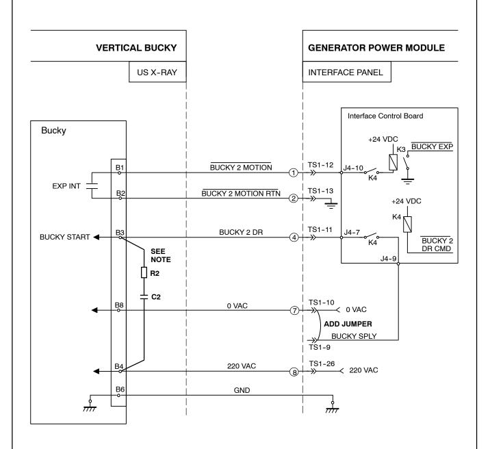
NOTE : In the case of noise due to Bucky, add R2=22 ohm, 1/2w, 5%; and C2=470 nF, 250 VAC as shown.
