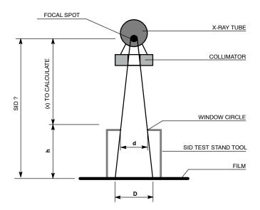
c. Measure the radius of the circle (**D/2**) obtained on the Processed Film *(refer to Illustration 4-14)*.
