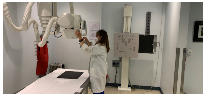
Virdin prepares the X-ray room for the next patient exam. South Lyon has one AeroDR HD flat panel detector in the wall bucky and another for the table.
