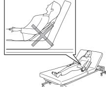
\* If the AeroDR Detector is placed on a sloping surface and subjected to a load, its internal sensor may be damaged.
