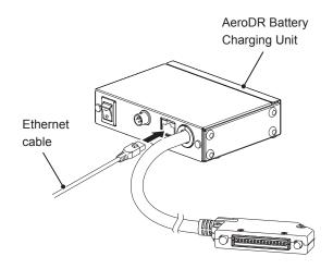
2 Connect the Ethernet cable connected to AeroDR Battery Charging Unit to the Hub.
